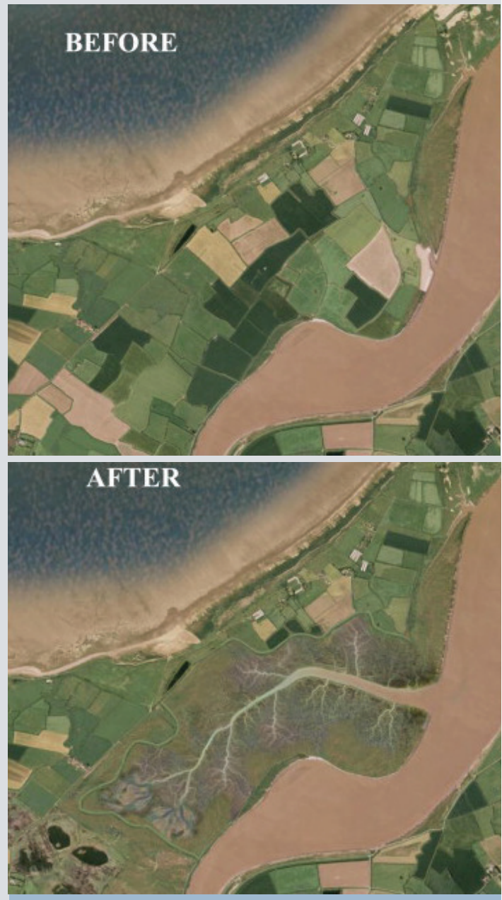
Restoration of low-elevation farmland to tidal marsh (i.e., “managed realignment”) can improve coastal resilience, provide valuable habitat for fish and wildlife, and offers many other public benefits. Vieira de Silva et al. (2014), used by permission of Elsevier
